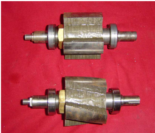
Fig. 9. Photo of the prototype rotors. Top: unskewed rotor. Bottom: skewed rotor.
