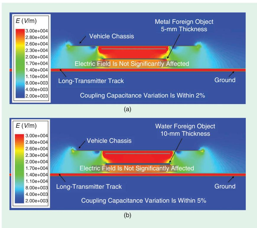
**Figure 10.** The impact of conductive and dielectric foreign objects on electric fields in a dynamic CPT system. (a) A metal foreign object and (b) a water foreign object.
