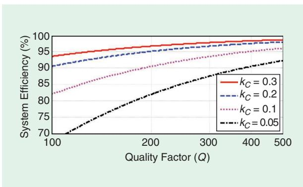
**Figure 6.** The efficiency of a CPT system at different coupling coefficient  $k_C$  and component  $Q$ .
