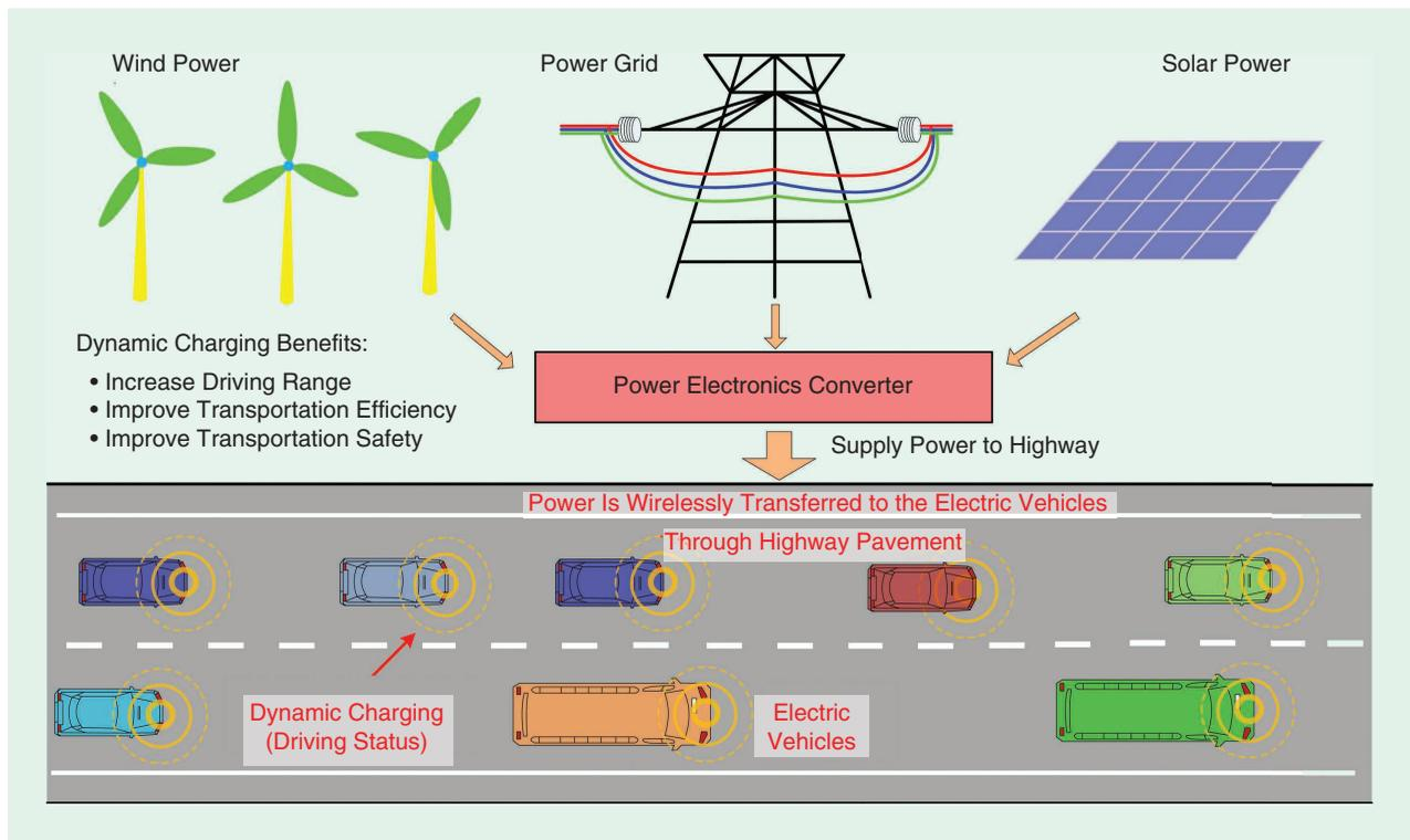
**Figure 1.** The electric roadway system with diverse renewable sources for electric vehicle charging applications.
