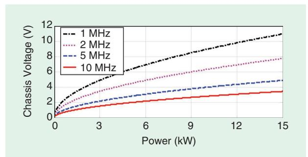
**Figure 7.** The chassis voltage at different power and frequency conditions. When the mutual capacitance  $C_M = 50$  pF, the chassis stray capacitance is 10 nF.
