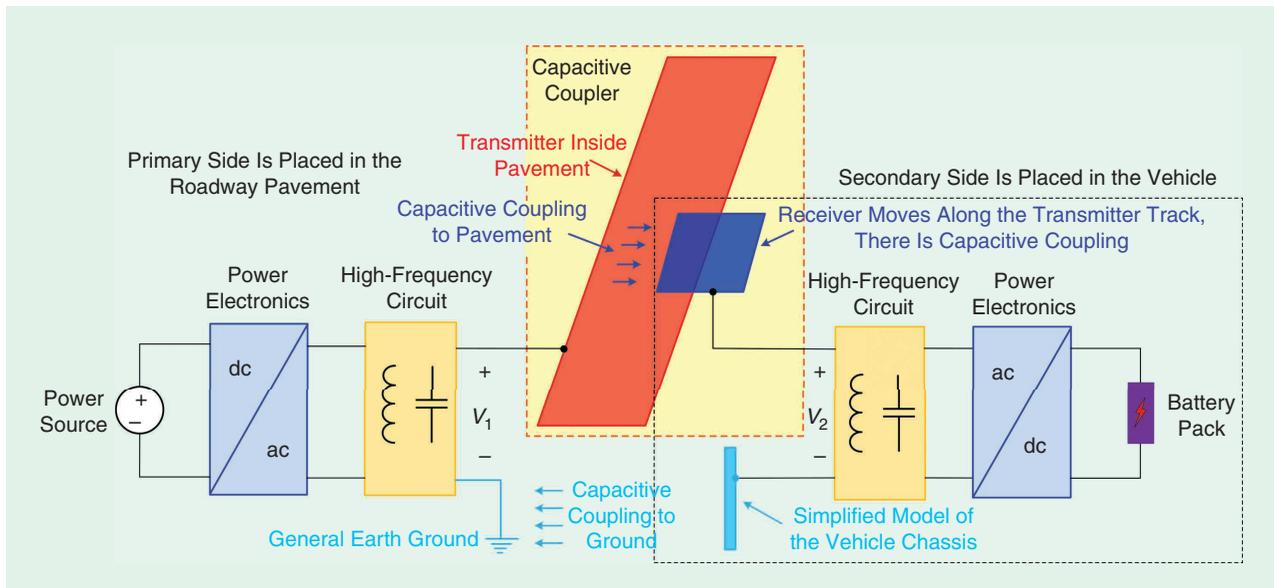
Figure 4. A simplified and equivalent circuit model used for an electric roadway system for dynamic charging.
