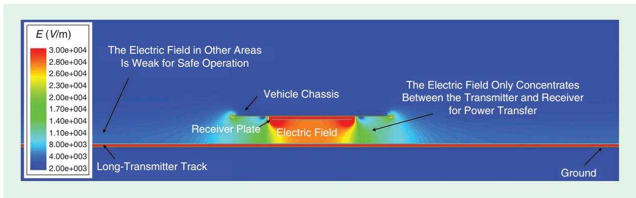
**Figure 9.** A simulated electric field distribution in a dynamic CPT system, demonstrating its safe operation.
