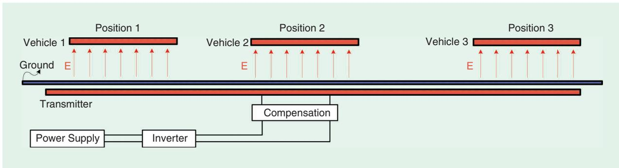
**Figure 12.** A long-transmitter track with multiple vehicles at different positions.
