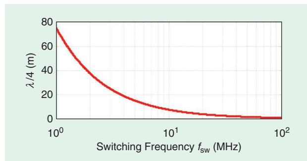
**Figure 13.** The relationship between switching frequency  $f_{sw}$  and quarter-wavelength  $\lambda/4$  of the electromagnetic wave.
