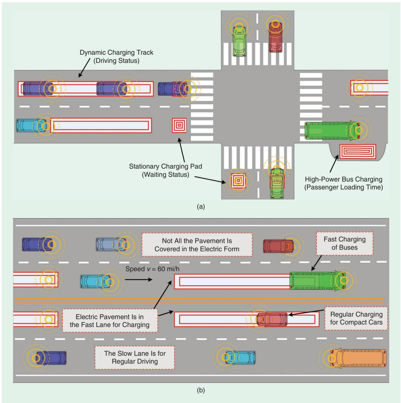
**Figure 11.** The practical implementation of the proposed electric roadway system used to achieve dynamic CPT charging for electric vehicles. (a) A low-speed electric roadway with a traffic light system and (b) a high-speed electric roadway on a highway system.
