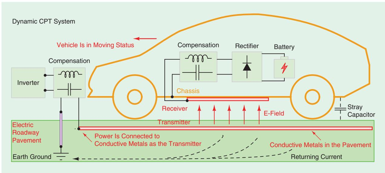
Figure 3. The structure of a dynamic CPT system for the electric vehicle charging application using electric fields.
