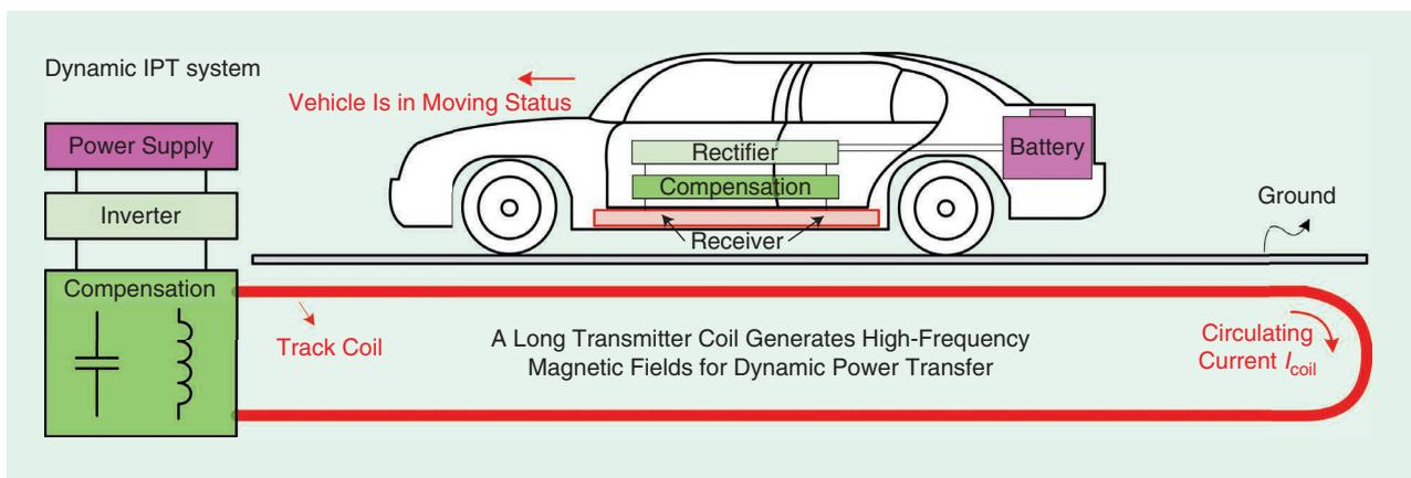
**Figure 2.** The structure of a dynamic inductive power transfer (IPT) system for the electric vehicle charging application using magnetic fields.
