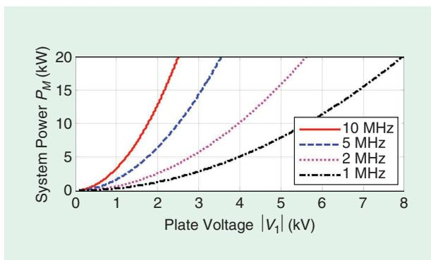
**Figure 5.** System power  $P_M$  at different voltage and frequency conditions when the coupling capacitance  $C_M = 50$  pF.
