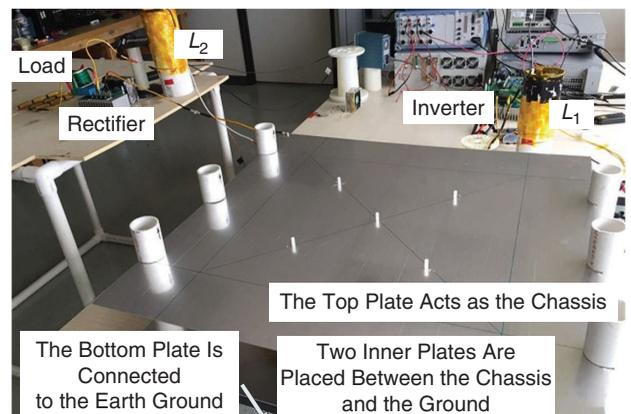
**Figure 8.** A lab-based prototype of a grounded CPT system used for high-power electric vehicle-charging applications.
