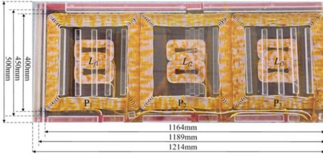
Fig. 10. Structure and dimension of primary transmitter coils  $P_1$ ,  $P_2$ , and  $P_3$ .
