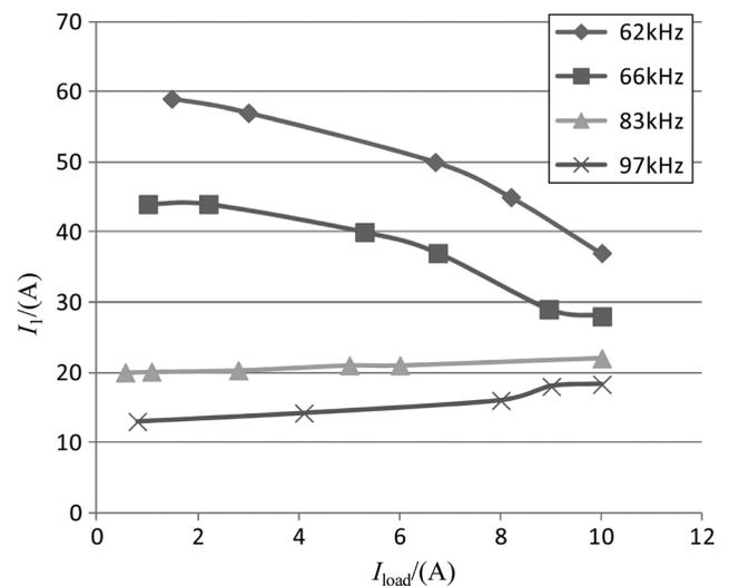
Fig. 7 Load-dependent property under different switching frequencies
