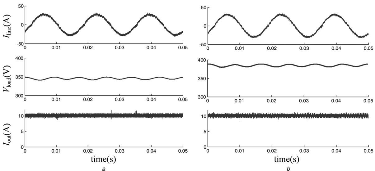
Fig. 9 LLC steady-state test as an on-board charger with various battery load  $I_{load} = 10 \text{ A}$ ,  $V_{in} = 200 \text{ V}$
