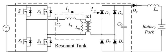
**Fig. 1** Schematic of a full bridge LLC converter
