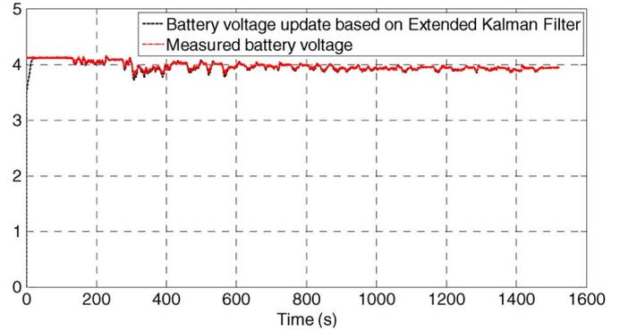
Fig. 21. Comparison of predicted and measured battery voltage.
