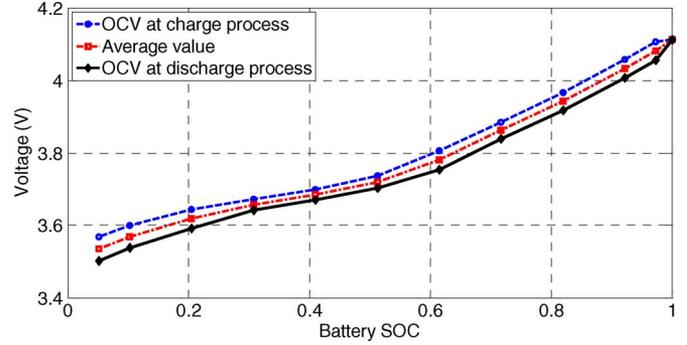
Fig. 3. Relationship between open circuit voltage and SOC.
