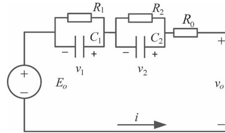
Fig. 2. Equivalent circuit model of the battery.
