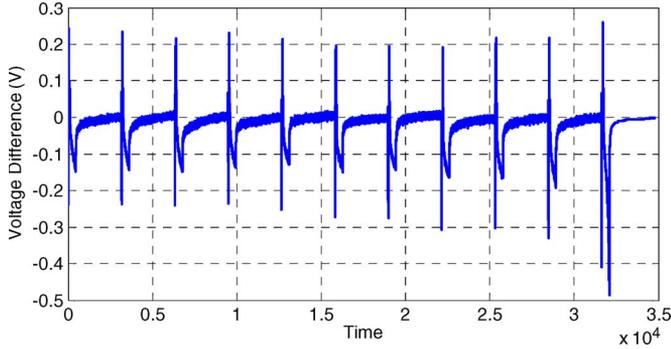
Fig. 5. Differences between battery terminal voltage and open circuit voltage.
