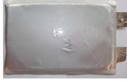
Fig. 1. Lithium-ion pouch battery cell used for a PHEV and the study in this paper.
