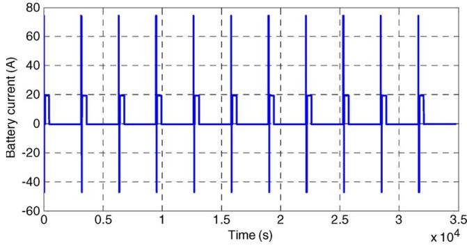
Fig. 4. Battery current profile for circuit parameter identification.
