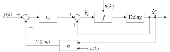
Fig. 9. Blok diagram of EKF calculation.
