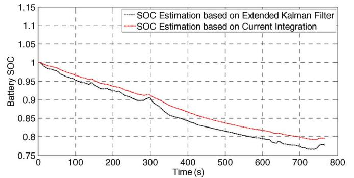
Fig. 16. Battery SOC estimation under HWFET drive cycle.
