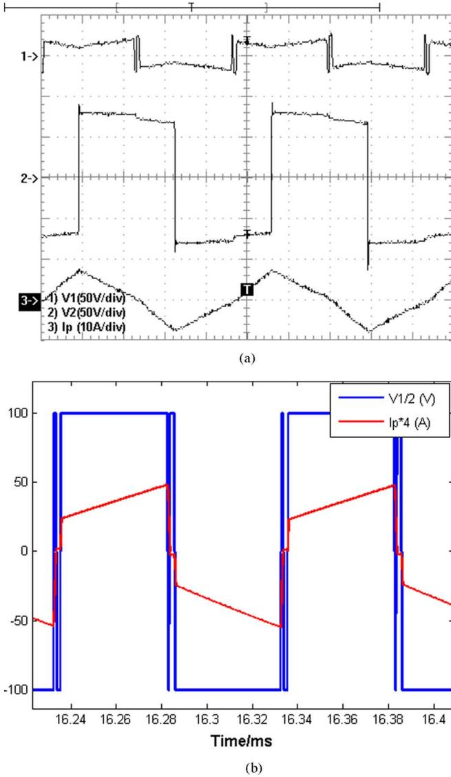
Fig. 2. Deadband effect on the primary voltage waveforms. (a) Experiment results. (b) Simulated results.
