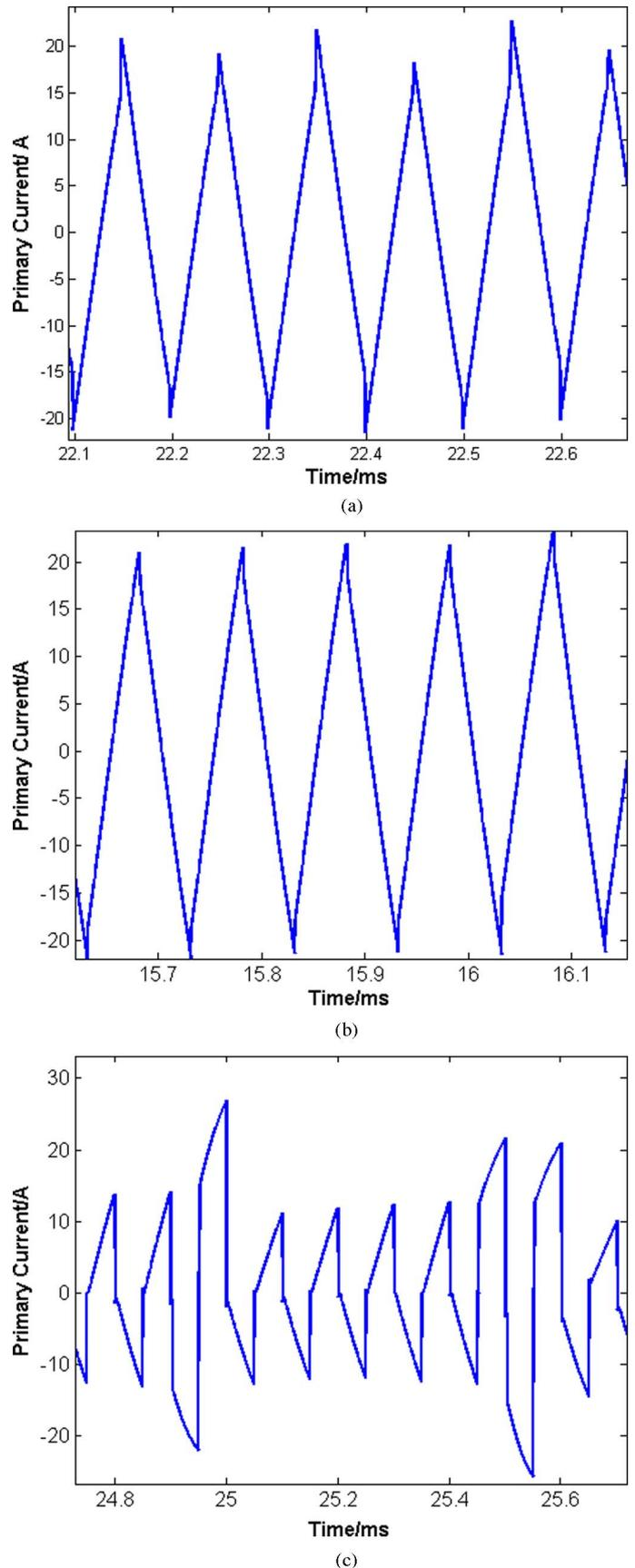
Fig. 12. Current under different turns ratio when  $V_1 = 200$  V,  $V_2 = 400$  V. (a) Turns ratio = 0.55:1. (b) Turns ratio = 0.47:1. (c) Turns ratio = 0.5:1.
