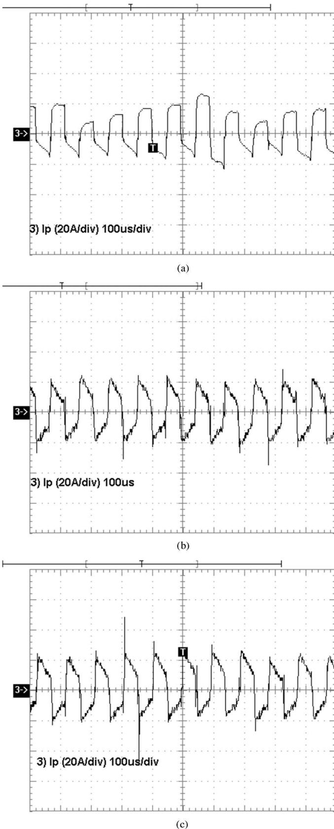
Fig. 13. Current under different inductance with  $V_1 = 200$  V,  $V_2 = 400$  V, and  $P_o = 5.1$  kW. (a) Current under single transformers. (b) Current under series-connected transformers. (c) Current under one transformer series with another leakage inductance.
