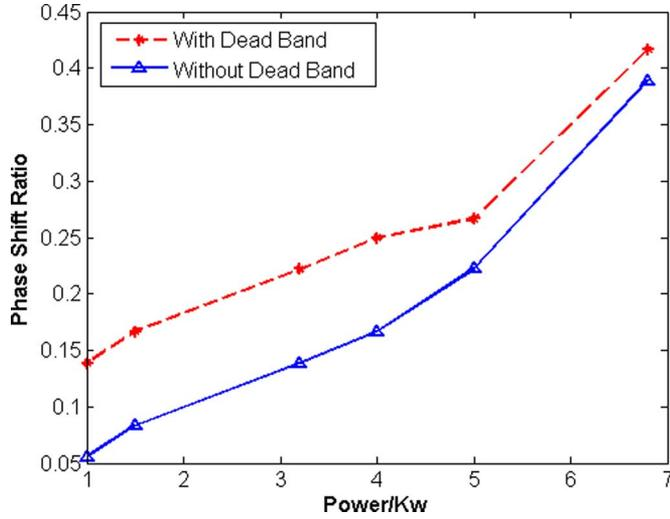
Fig. 9. Comparison of phase-shift angle in the steady state to maintain constant output voltage (simulation).
