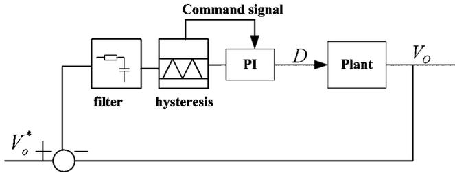
Fig. 11. Proposed schematic to erase the shift error.
