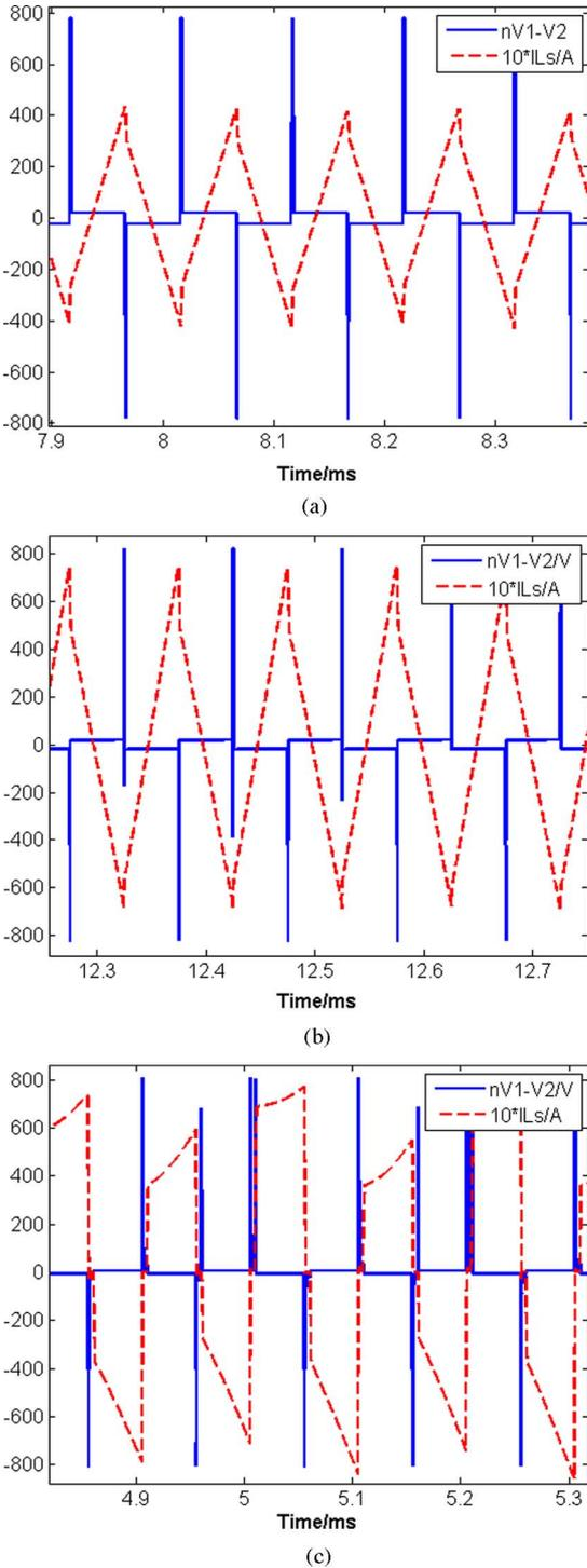
Fig. 5. Current waveforms under different operation modes. (a)  $V_1 = 200$  V,  $V_2 = 380$  V. (b)  $V_1 = 200$  V,  $V_2 = 420$  V. (c)  $V_1 = 200$  V,  $V_2 = 400$  V.
