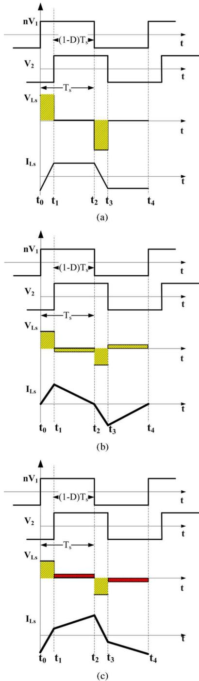
Fig. 3. Operation modes of phase-shift control under different output voltage. (a)  $V_2 = nV_1$ . (b)  $V_2 > nV_1$ . (c)  $V_2 < nV_1$ .
