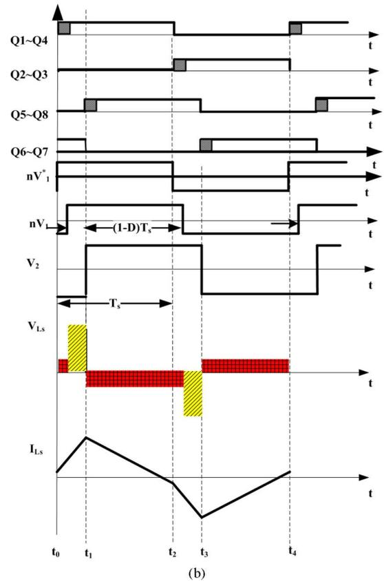
Fig. 10. Influence of deadband to the phase shift under different load conditions. (a) Phase shift under heavy load with deadband ( $I(t_0) < 0$ ). (b) Phase shift under light load with deadband ( $I(t_0) > 0$ ).
