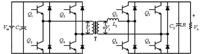
Fig. 1. Isolated bidirectional dc–dc converter system in an HEV.
