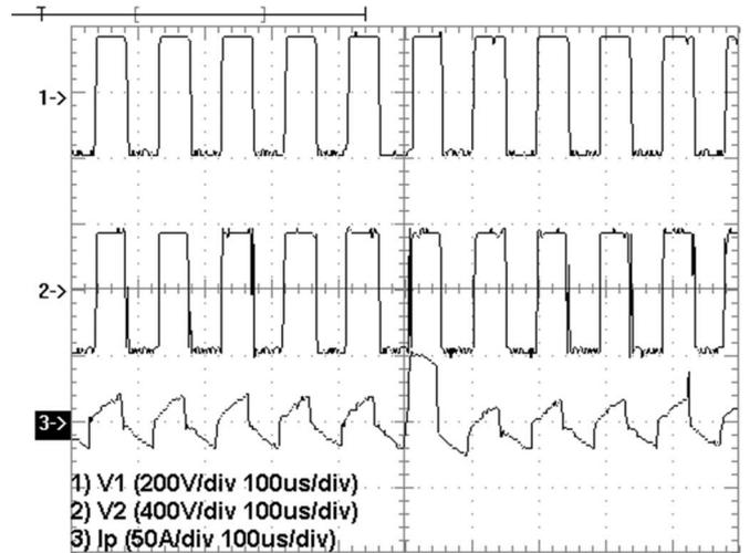
Fig. 4. Pulse sequence when current varies near  $nV_1 = V_2$ . (Channel 1  $\rightarrow$   $V_1$ , Channel 2  $\rightarrow$   $V_2$ , Channel 3  $\rightarrow$   $I_p$  (primary current)).
