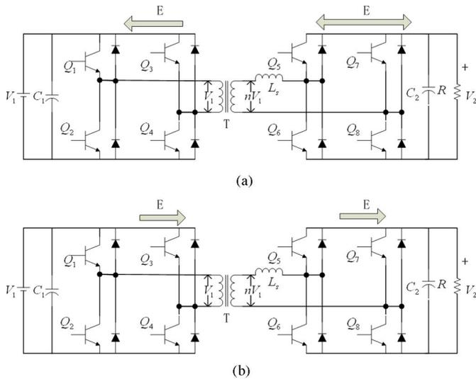
Fig. 7. Energy flows in the different stages with the consideration of deadband effects. (a) Energy flows during interval  $db_1$ . (b) Energy flows during interval  $\Delta D$  and  $db_2$ .
