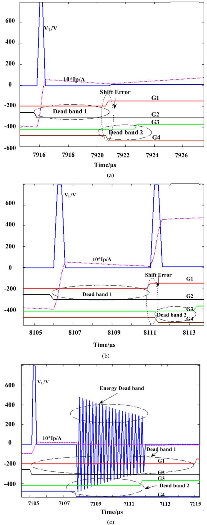
Fig. 6. Current variation caused by different time sequence of  $G_1$ – $G_4$ . (a) Details where current is small in Fig. 5(c). (b) Details where current is large in Fig. 5(c). (c)  $nV_1 = V_2$  when  $P = 400$  W.
