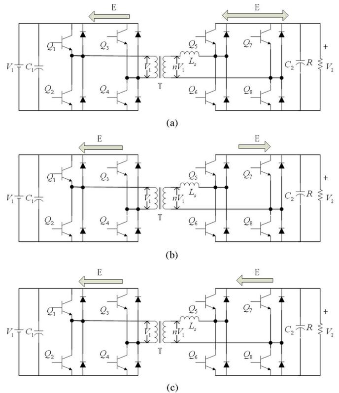
Fig. 8. Energy flow in the very light load when  $db_1 > db_2$ . (a) Energy flow during interval  $\Delta_1$ . (b) Energy flow during interval  $db_2$ . (c) Energy flow during interval  $\Delta_2$ .
