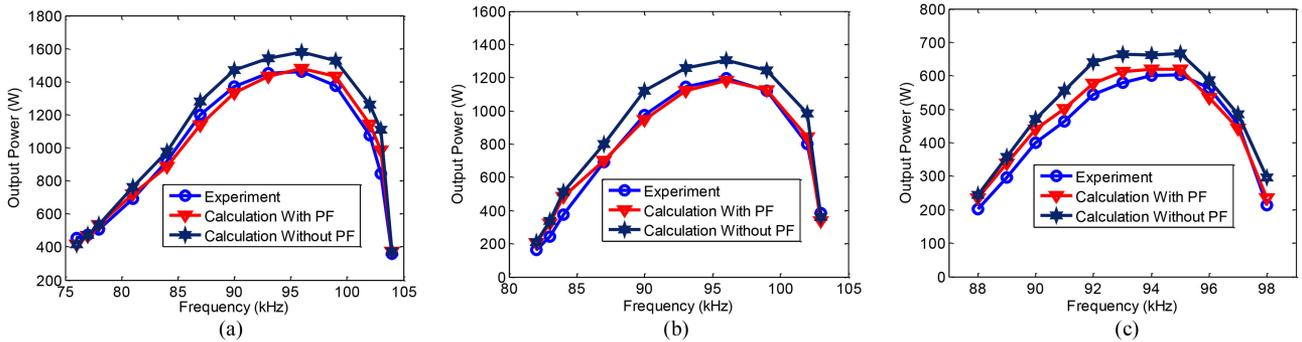
Fig. 14. Experimental and calculated output power of the WPT system at different frequencies. (a)  $X = 0$  mm,  $Y = 0$  mm. (b)  $X = 200$  mm,  $Y = 0$  mm. (c)  $X = 0$  mm,  $Y = 150$  mm.
