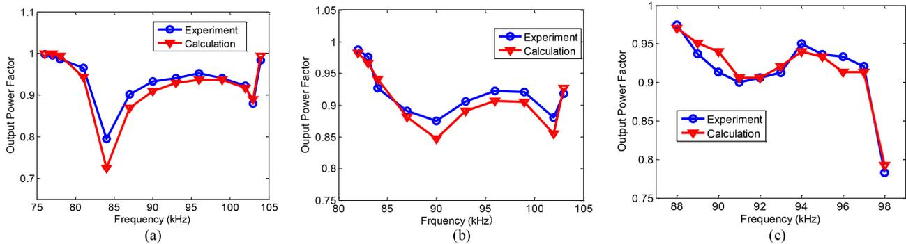
Fig. 11. Experimental and calculated ac output power factor of the WPT system at different frequencies. (a)  $X = 0$  mm,  $Y = 0$  mm. (b)  $X = 200$  mm,  $Y = 0$  mm. (c)  $X = 0$  mm,  $Y = 150$  mm.
