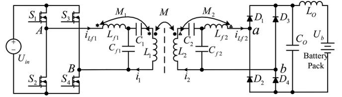
Fig. 1. Studied integrated *LCC* compensation topology.
