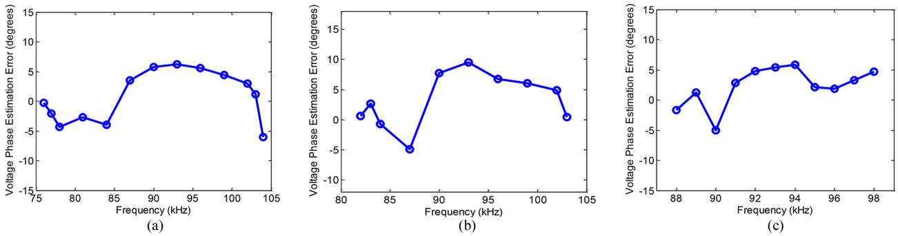
Fig. 13. Estimation errors between experimental and calculated results of input and output voltage phase difference at various frequencies. (a)  $X = 0$  mm,  $Y = 0$  mm. (b)  $X = 200$  mm,  $Y = 0$  mm. (c)  $X = 0$  mm,  $Y = 150$  mm.
