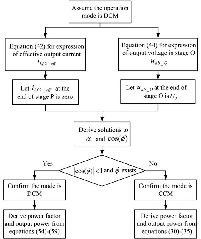
Fig. 6. Flow chart for mode identification and parameter derivation.
