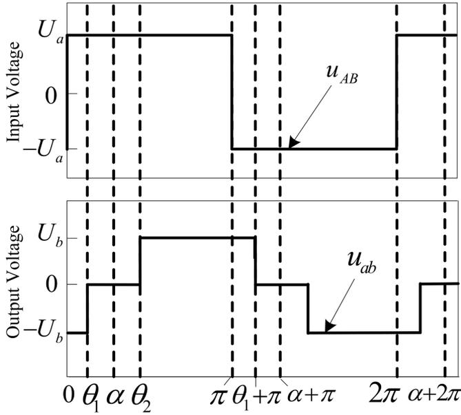
Fig. 5. Equivalent voltage waveforms of DCM.
