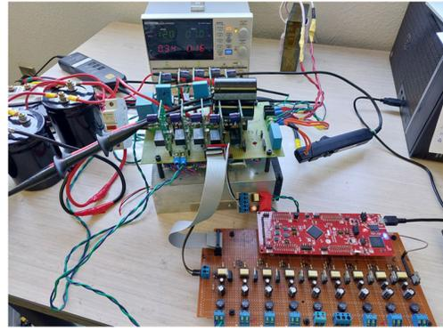
Fig. 5. Experimental setup for file-level proposed inverter.
