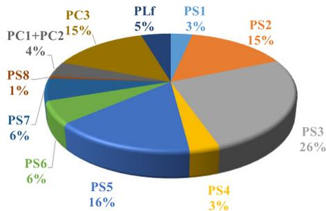
Fig. 11. Loss breakdown of the proposed inverter.
