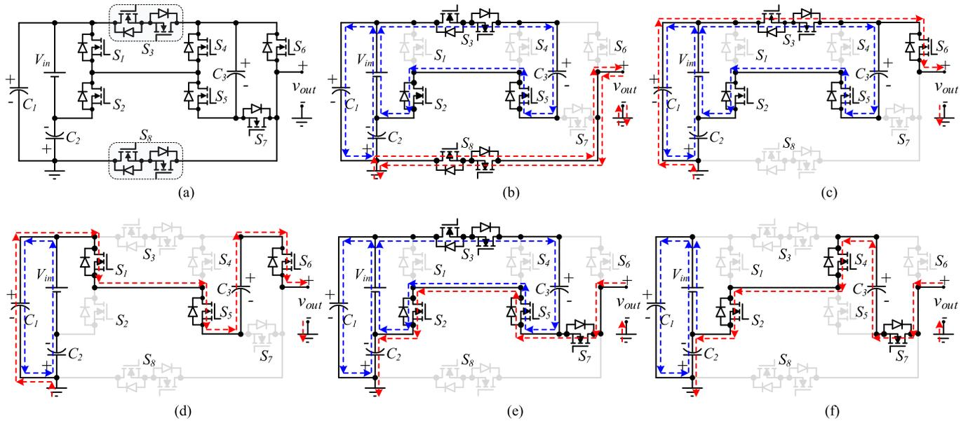
Fig. 1. Proposed five-level inverter and its operating modes. (a) Proposed topology, (b) first mode,  $v_{out} = 0$  V, (c) second mode,  $v_{out} = +0.5V_{in}$ , (d) third mode,  $v_{out} = +1.5V_{in}$ , (e) fourth mode,  $v_{out} = -0.5V_{in}$ , and (f) fifth mode,  $v_{out} = -1.5V_{in}$ .
