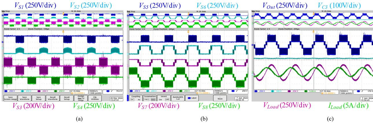
Fig. 7. (a) Voltage stress of switches  $S_1$ – $S_4$ , (b) voltage stress of switches  $S_5$ – $S_8$ , and (c) nonunity power factor load conditions: output voltage of inverter before filter, the voltage of capacitor  $C_3$ , load voltage, and load current with a phase difference of more than  $80^\circ$ .
