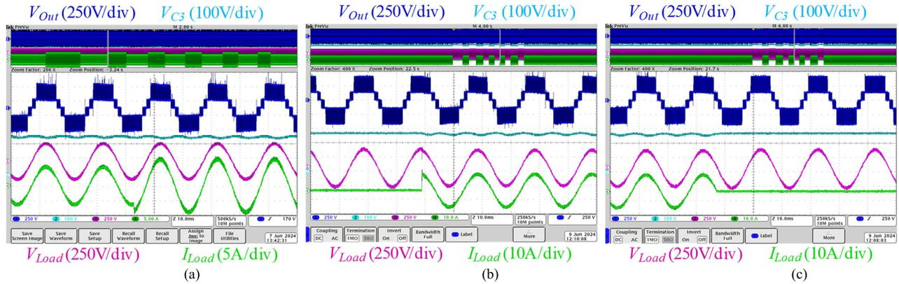
Fig. 8. Output voltage of the proposed inverter before the filter, voltage of capacitor  $C_3$ , load voltage, and load current during a step change in the output power. (a) Step change in the output power from 1.14 to 1.6 kW, (b) step change in the output power from 0 to 2 kW, and (c) load change from full power (2 kW) to 0.
