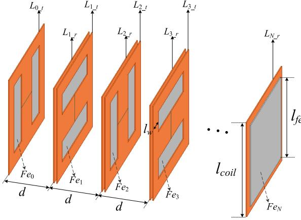
Fig. 3. Coil structure of the proposed WPT system.
