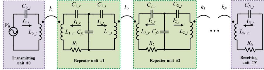
Fig. 2. Structure of the proposed multi-load WPT repeater system.
