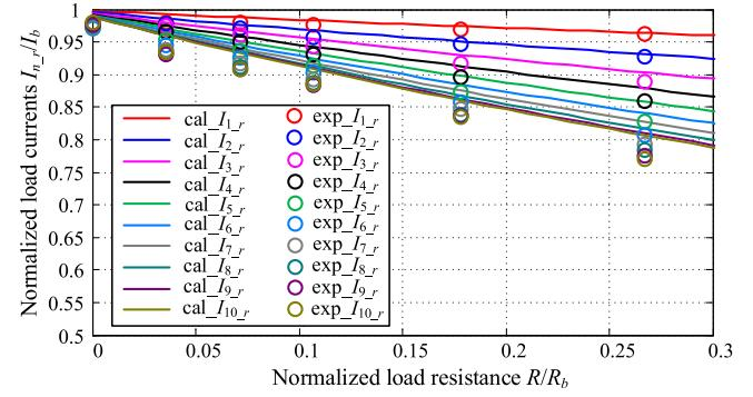
Fig. 7. Load current variation against the load resistance.
