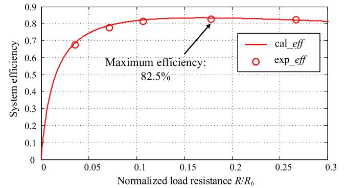
Fig. 8. System efficiency of the experimental setup ( $k = 0.24, Q = 280$ ).
