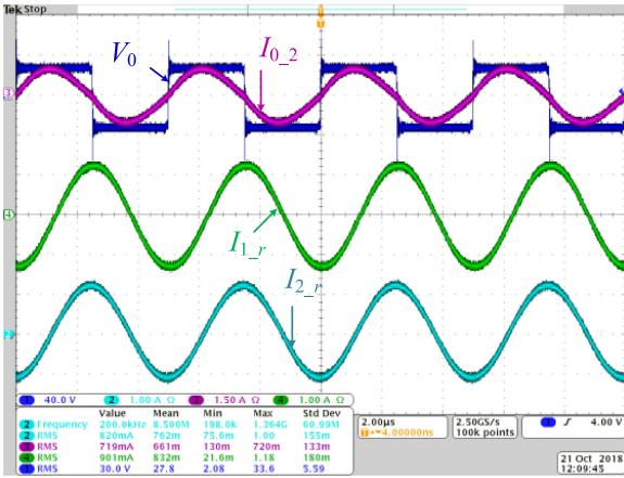
Fig. 5. Experimental waveforms of the voltages and currents.
