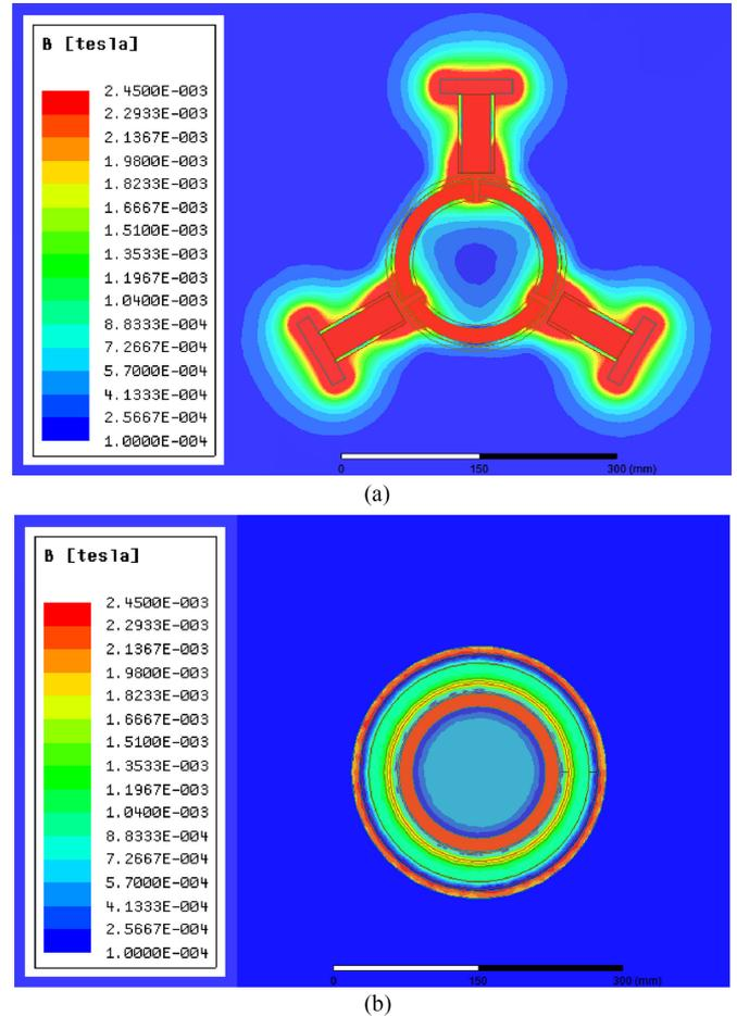
Fig. 6. Magnetic flux densities in YZ plane: (a) proposed coil structure and (b) coaxial coil structure.
