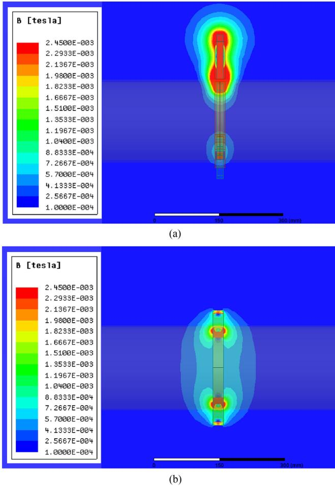
Fig. 7. Magnetic flux densities in ZX plane: (a) proposed coil structure and (b) coaxial coil structure.
