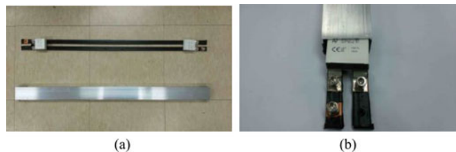
Fig. 7. Aluminum box and capacitor banks for the S-type power supply modules [71]. (a) Separated case. (b) Inserted case.
