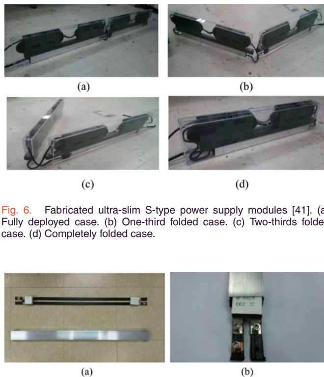
Fig. 7. Aluminum box and capacitor banks for the S-type power supply modules [71]. (a) Separated case. (b) Inserted case.
