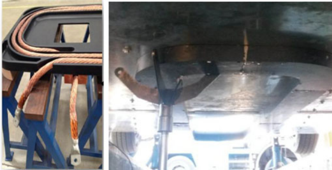
Fig. 19. U-type power rail (left) and rectangular pick-up (right) used for the RPEV developed by the VICTORIA project [87].
